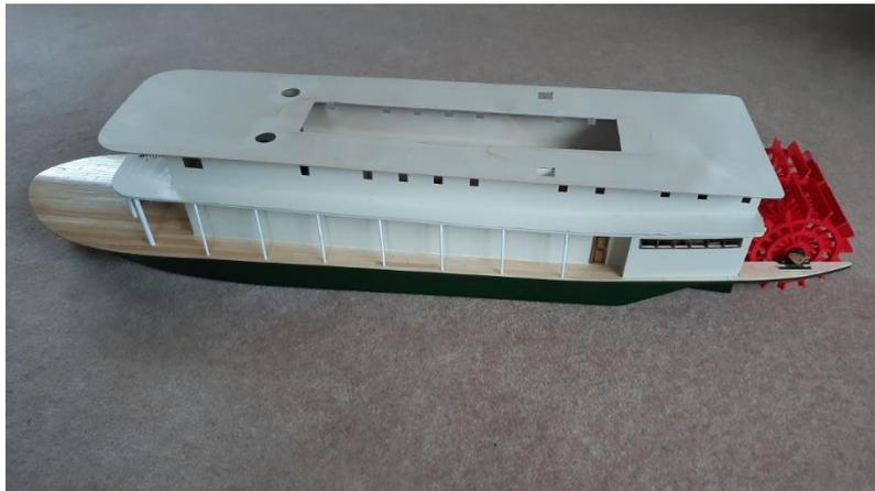
The rest of the summer and autumn were spent building up the superstructure, spraying and adding details as I went. I finished laying out the electrics including adding connectors for the wiring to make it easy to change at a later date if needed. I modified some of the staircase designs as I went to match the space available to fit them.
