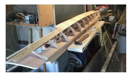
I used a 150mm x 20 mm timber base board cut to the length of the model, and this was used as a construction 'jig' which allowed the 14 model frames to be aligned and glued accurately to the keel, stem and stern. The centre of the frames were cut out using a jigsaw.
