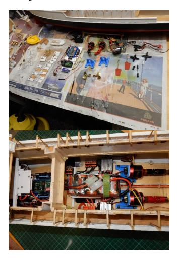
The target weight was about 3.6 to 4kg. Originally I had a trial run at the pond, after Lockdown 2, before #3, and found the optimum weights, and trims, with a 7.2V NiMH battery. But the boat is too fast!
