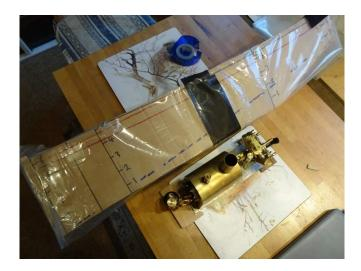
It took quite a lot of running in, dismantling and adjusting, to get it to run smoothly. I have also added a small glass jar to serve as a separator with an alloy pipe from the exhaust and an outlet running up the side of the ornate funnel. This prevents a mixture of scalding oil and steam being sprayed about over the passengers and crew somewhat lessening the pleasure of their voyage!
