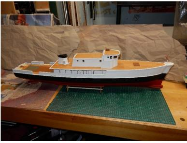
Most of what happened next was the deck fittings. The main mast is removable, and I drilled through the main deck and forward part of the lower deck, gluing in larger diameter plastic tubes. I changed the wooden masts for plastic, as I could then run the cables for the lights and radar motor, inside these tubes. I have used a mix of motor/transformer windings, and some 32AWG wire. The radar motor is again a Precision Micro drives 6mm diameter, 22mm long, 43 RPM geared motor.
