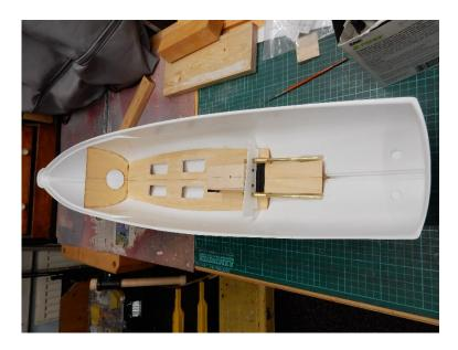
The round hole in the front bulkhead could have been larger, as the space is almost inaccessible, once the main deck goes on. I wanted to put lights in the bow windows, but wasn't too clever with my soldering and had to patch the hull where it got too warm!
