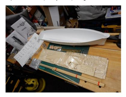
The instructions have a few words about the original "Calypso," but there are no words to show the process of putting everything together. The design is aimed at a display model, so some modifications are relevant to making a working model. I changed the propeller shaft design (for Raboesch waterproof ones,) and replaced some of the brass work, particularly those on higher deck levels, for stability.
