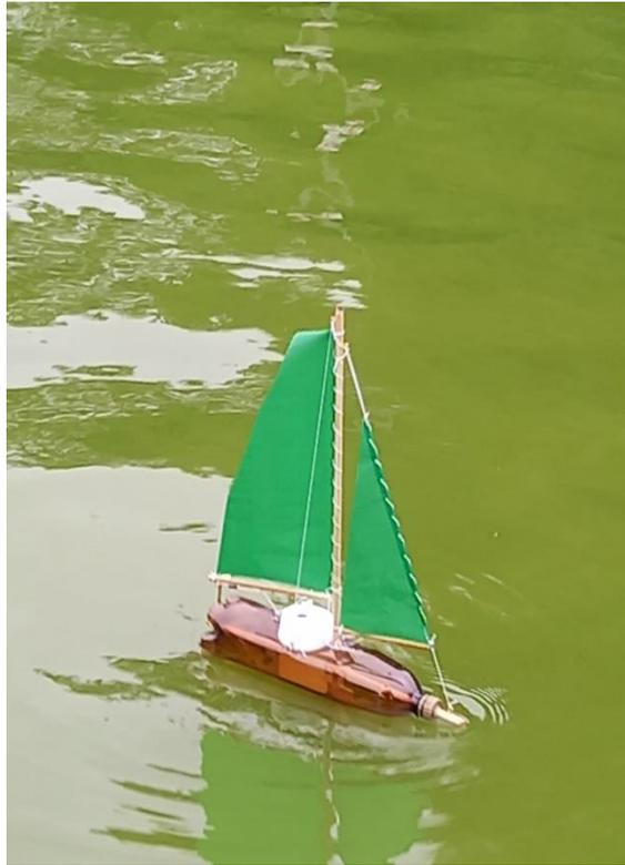
Would I change the design to make construction easier? Yes, you only find out by making mistakes and I am still not sure if you need the structural dowel going through the bottle. I would also fit the mast through the bottle and glue the dagger board onto it to save cutting the slot.
