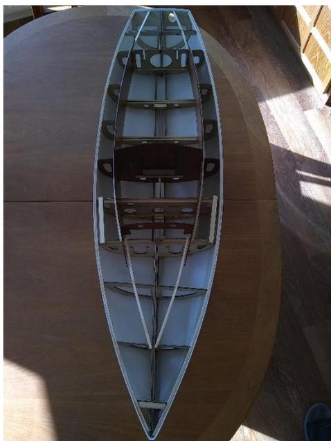
With all deck stringers installed the centreboard, after being spray painted a copper colour, was glued into place using Araldite to make a hopefully waterproof seal. The model requires an additional 1.5kg of ballast and after a long internet search loose lead shot was located on eBay at a reasonable price and 2kg have been ordered with delivery due in the next couple of days.
