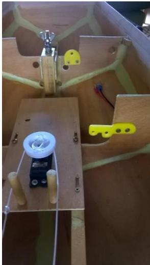
Plastic guides were fitted to stop the sheets from tangling and the rudder support was glued in place. Yellow Milliput is clearly visible on the seams.
