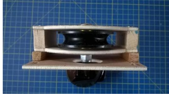
The sail control consists of a drum servo towards the stern and a plastic pulley wheel at the bow giving a loop of about 18 inch length.
