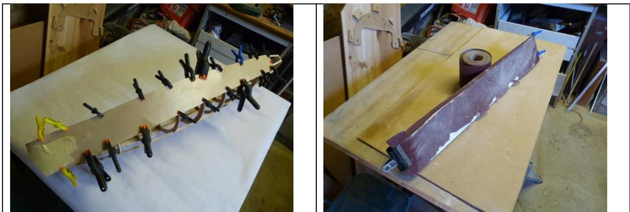
Now it's time to glue the sides on. This was made easy due the flat sides of the design that only required a single sheet of ply and lots of clamps, but you have to be careful that the ribs and frame are flat for total coverage of the glue. To achieve this flatness I use a long flat board and a length of abrasive paper with clips at either end which is nearly as long as the boat. This helps to remove any high spots over a long length easily.
