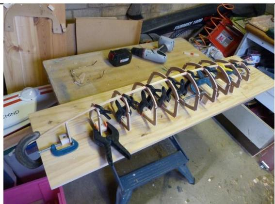
To hold the ribs square and in line a flat ridged base board was used, the blocks being screwed squarely to each other at the spacing specified by the drawing.
