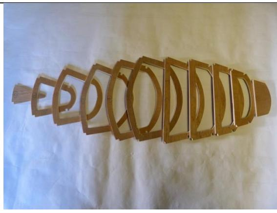
I finished the outside using files. To keep the boat light the centres were cut out using a jig saw and files. Also shown are the notches because I was going to make a frame to glue the planking against.
