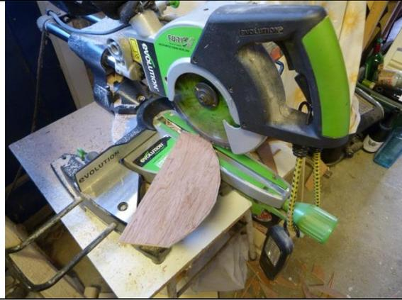
I photocopied the rib section 10 times (10 ribs on this model) then cut out each one to act as a pattern. You have to fold each one in half as the drawing only shows half the rib before cutting. This also allows you to get both halves the same. Because I only have hand tools, except a saw and drill, I cut the outside with a chop saw.
