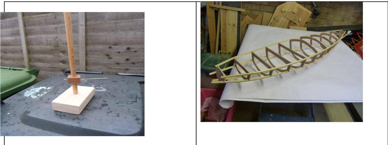
I made a depth pointer to help with keeping the frame square. This was used when on and off the jig during the build.
