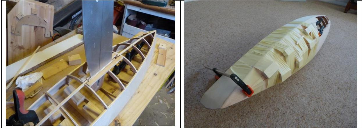
As I had a sheet of Alloy in the garage I made the dagger board from it, but still cut to the ordinal shape. I made a special frame as the one shown on the drawing was for a thicker, removable dagger board as in the 1 metre regulations. The base can now be glued on with lots of masking tape and blocks to hold the planks against the frame. At this point I admit that I made a mistake by not using narrower planks on the bottom but you always learn by your mistakes.
