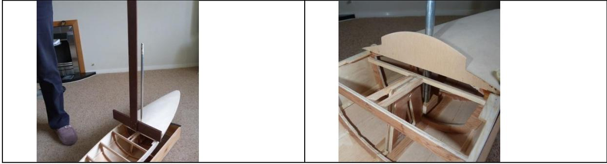
Squaring up the mast before gluing the support tube and base block in place. Using this method the mast just drops into the tube for easy transport.
