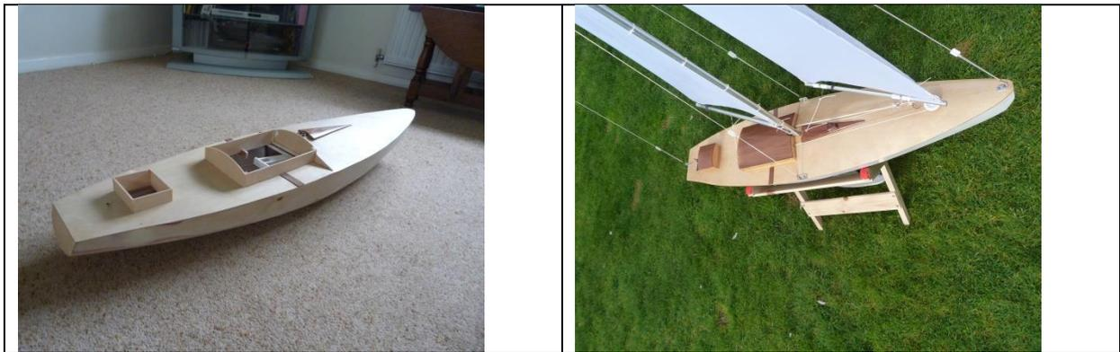
Rear deck fitted and glued in place. At this time I decided to add cabins to the rear deck and make it into a 1930 type sailing yacht. I decided not to use the normal sticky plastic racing pads as I was not going to be racing and wanted the craft to look different on the water.
