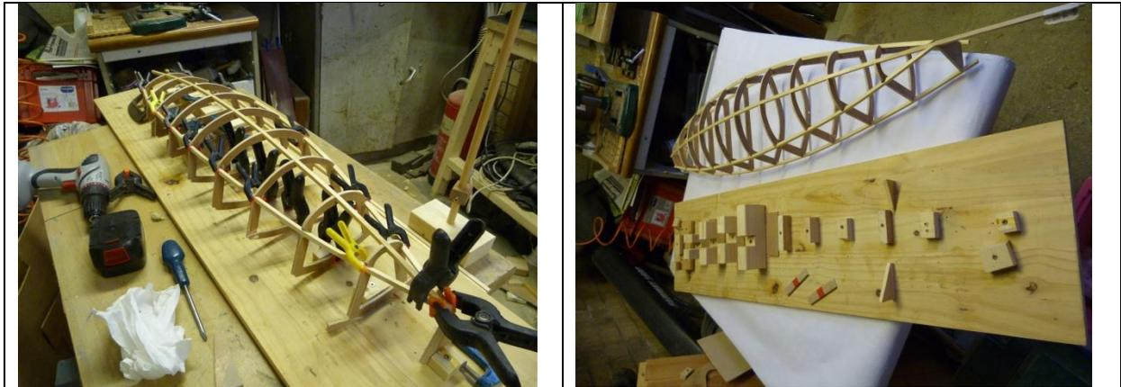
After gluing the assembly can be lifted off the jig and checked for squareness. It's better to check at this stage when adjustments can be made by cutting and regluing.
