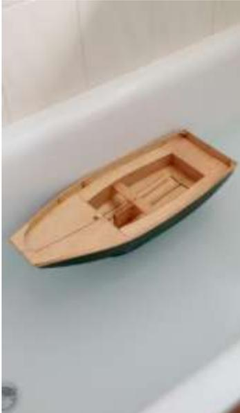
Following fitting of the dagger board keel and lead bulb weight, which were fixed by using fast setting epoxy glue, it was time for initial flotation tests using the bath.
