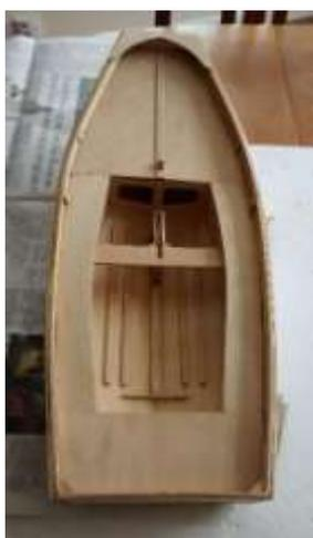
After a bit of fettling decks were installed along with rigging plates, mast step and other parts. These were then varnished, in total some 10 coats of satin finish varnish was applied to the boat's interior.
