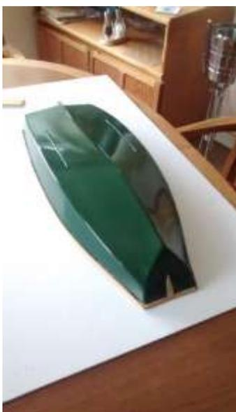
Halfords car body grey primer spray paint was used and after at least 24 hours drying per coat, the surface was rubbed down with fine grit. Almost 2 cans were used to provide the 6 coats applied. The colour coat was the applied again using Halfords spray paint in Brookwood Green. At least 48 hours drying time was allowed before rubbing down each coat with fine grit. 8 colour coats were applied.
